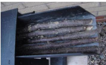
Use the scraper to form a bridge half way along the wood tray. Place sticks on the scraper with the ends protruding into the firebox.
