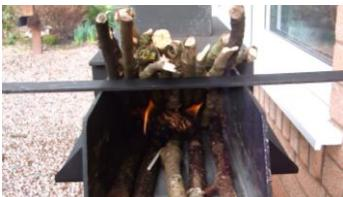
When the sticks are burning well, remove the scraper while supporting the sticks as shown.
