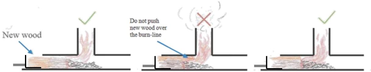
You need to keep the fire burning in a straight line. If it starts to burn along one side of the stack faster than the other side or along the bottom faster than the top, carefully adjust the stack until the burn-line is even again. If you always place the larger sticks on the bottom of the stack, the burn-line will remain consistent.
