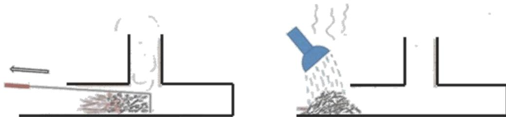
Separate any un-burnt wood from the biochar; dry it and keep it for next time.
